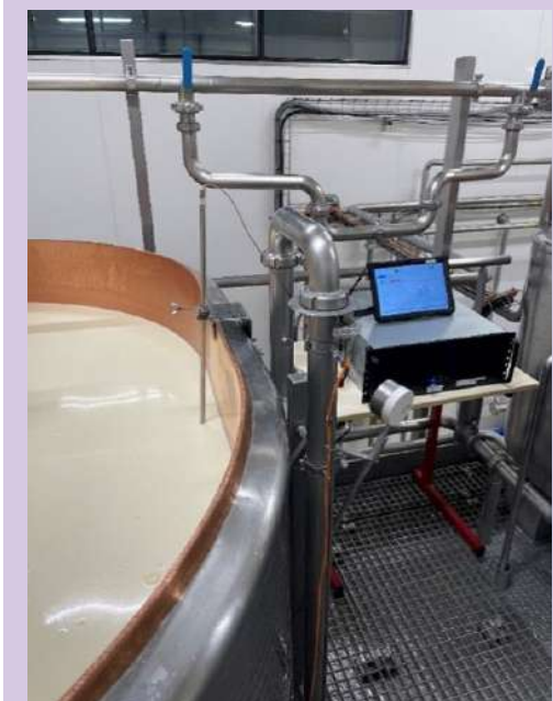
Acquisition and visualisation of coagulation curves during Comté cheese production. The sensor at the end of the rod is immersed in an 800-litre Comté vat.
