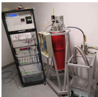
Cryogenic Saphir Oscillateur at the ESA Deep Space Antenna in Malargüe (Ar)
