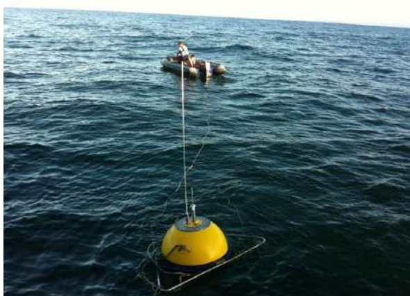
Waverider buoy which will be adapted for WAVEMEASUREMENT project
