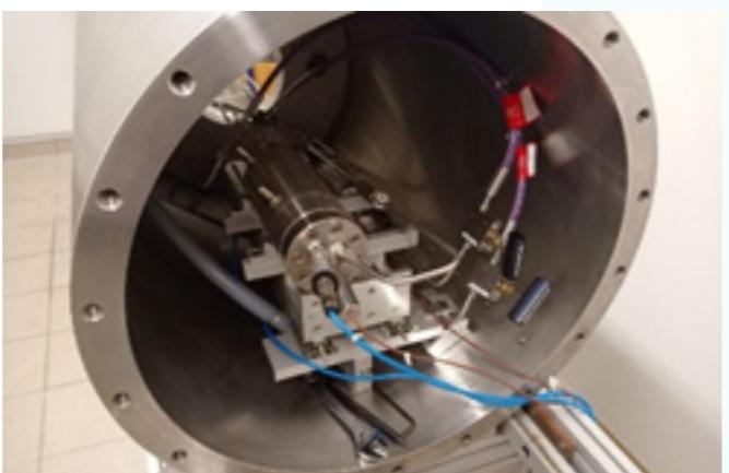
H<sub>2</sub> high-pressure pressurization chamber to promote damage to materials used in Type 4 tanks.
