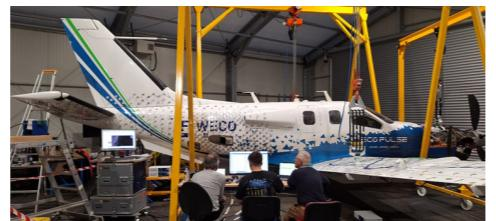
Setting up vibration tests on the ECOPULSE hybrid demonstrator.
