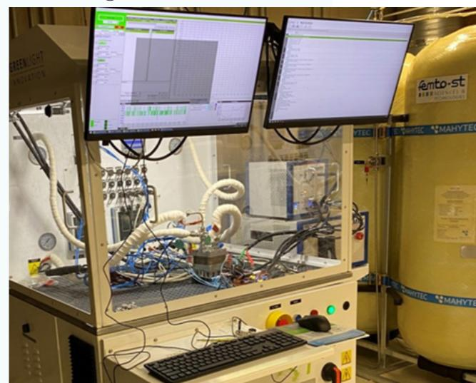
PEM Water Electrolyser Test Bench
