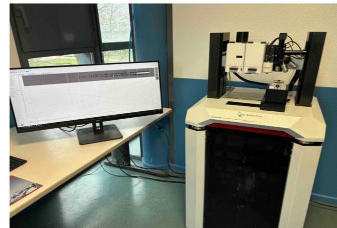
The Step500 platform produced by Anton Paar, available on the SURFACE platform, and equipped with an NHT3, NST3, and MCT3 indenter and an optical microscope.
