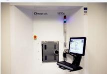
Features: ICP power source: 5.5 KW Bias power source: 1.5 KW Dual source Process temperature: 0 to 40 °C Clamping chuck: Electrostatic
