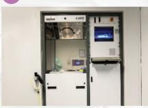
Features: ICP power source: 2 KW Bias power source: 0.5 KW Process temperature: -20 to 30 °C Clamping chuck: Mechanical Gas: SF<sub>6</sub>, C<sub>4</sub>F<sub>8</sub>, O<sub>2</sub>
