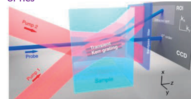
Principle of the transient grating induced by an infrared pump pulse in a transparent dielectric. The signal is generated by diffraction on the pump-induced transient grating and appears clearly in the far-field.
