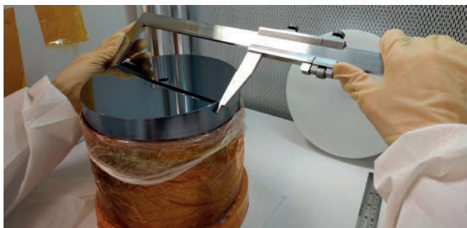
14 kg, 18 cm long single-crystal silicon cylinder that will constitute the spacer of a sub-1 K Fabry-Perot cavity. Optical contacting attachment of the cavity mirrors will be performed at FEMTO-ST.
