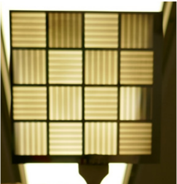
Silicon tool created specifically for ion implantation, 15 µm wide through holes spaced 15 µm apart, 380 µm deep.
