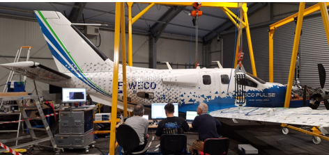
Setting up vibration tests on the ECOPULSE hybrid demonstrator.
