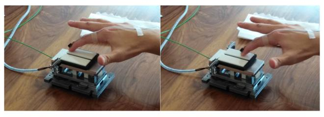
Figure: Example of a custom-built tribometer (© ECTO team, FEMTO-ST Institute) measuring mechanical signals at the interface between a finger and a solid surface. No such apparatus exists to study tactile interactions with soft or complex materials. Louyot et al., Tribology International 2024.
