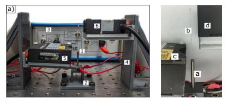
Left figure: 1. Piezoelectric tube actuated optical fiber; 2. Support base; 3. Voltage amplifier; 4. Sensors bases; 5&6. Displacement sensors. Right figure: a. Piezoelectric tube actuator; b. Optical fiber; c&d. Displacement sensors (the same as 5&6 in left figure)
