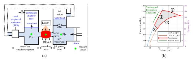
Figure 1: (a) Experimental setup of a flowloop that mimics the cardiac circulation, where 'DEAA' represents the tubular DEA [3]. (b) Measured pressure-volume relation without and with DEAA [3].
