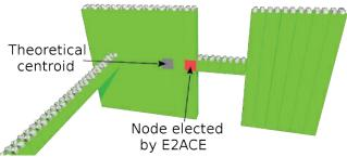
Example of the determination of the central node (Node elected by E2ACE) in a tridimensional network of microrobots.
