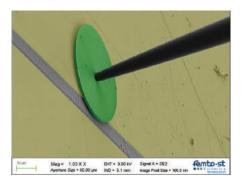
Scanning Electron Microscope image of the µdisk being aligned to a waveguide by a robotized tip.
