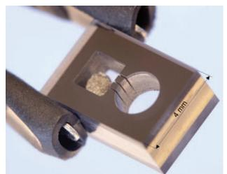
Single Cesium vapor cell fabricated at Tronics Microsystems.
