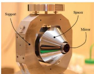
Picture of the optical frequency reference used to stabilize a laser: 140-mm long single crystal silicon Fabry-Perot cavity in its quasi-octagonal support.
