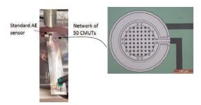
Left: A network of about 50 CMUTs installed on an aluminium plate; Right: A close-up of an individual CMUT.
