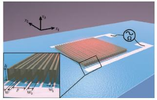
Schematic representation of the principle of the nanoscale acousto-optical modulator.
